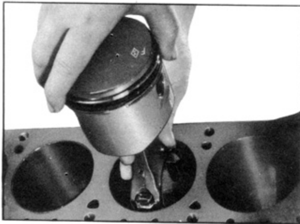
Removing Connecting Rod with Piston
